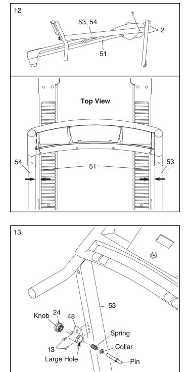
Attach the Latch Housing (48) to the Left Upright (53) with two #10 x 1" Tek Screws (13); start both Tek Screws, and then tighten each of them. Make sure that the large hole in the Latch Housing is on the indicated side.
